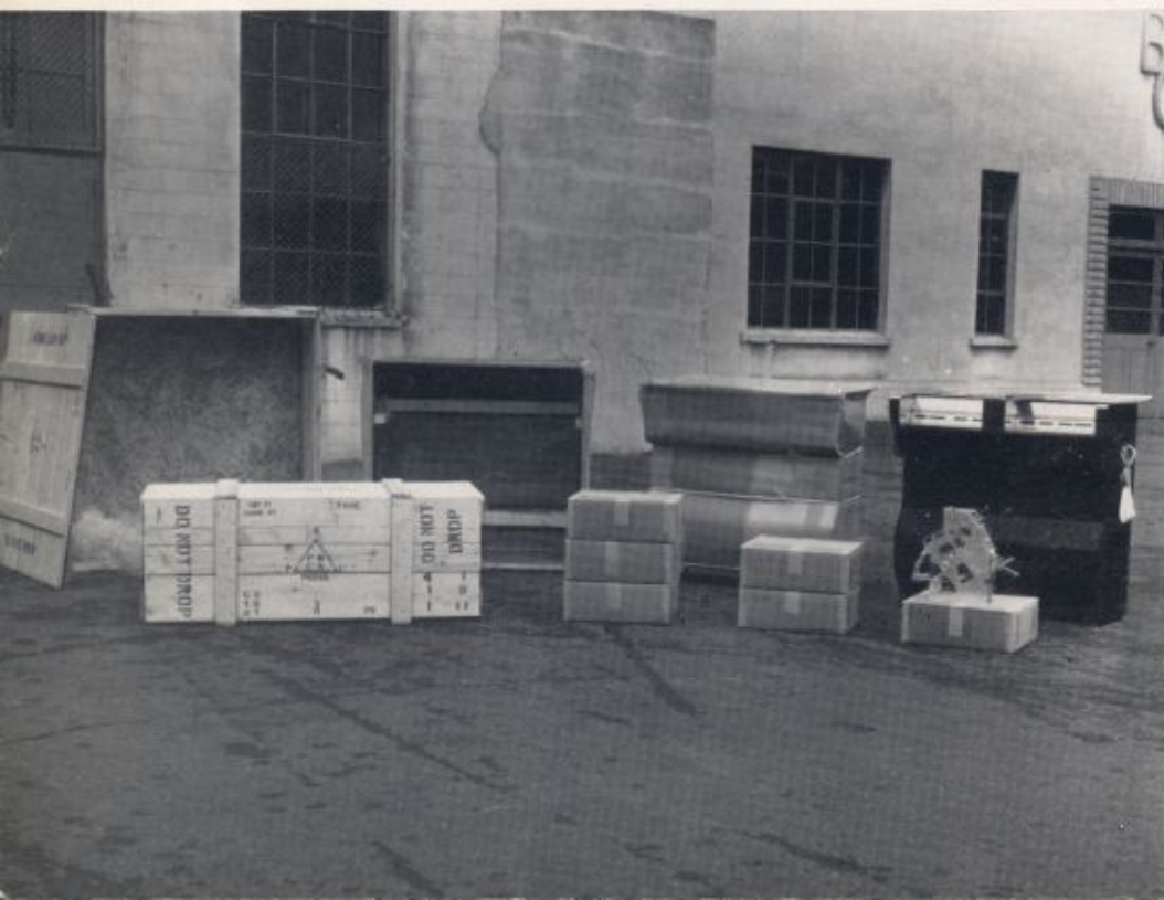
Progressive packing stages of an "S.P." machine for the Paris Metro with the casework at the rear and the unit mechanism at the front.
