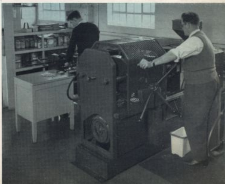
The nylon moulding equipment.
